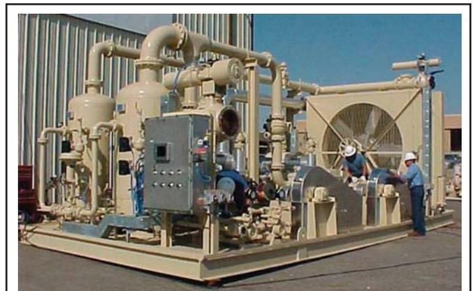
Vapor recovery units are designed to capture high-Btu content vapors that would otherwise be vented to the atmosphere, and turn them into a valuable revenue stream while simultaneously minimizing regulatory and liability exposures.
