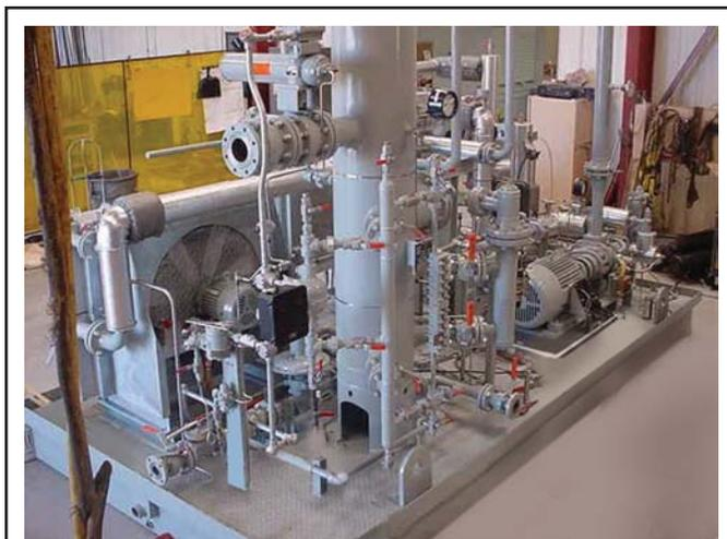
The compressor is a critical element in VRU system design. Rotary screw or rotary vane compressors are best suited to vapor recovery applications because of their ability to effectively handle wet gas. Shown here is a VRU installed on an offshore platform.
