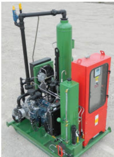
■ This OTA 24NG VRU is designed for locations without access to electricity. The package includes OTA's KS40 reciprocating compressor driven by a 23.5 hp (17.5 kW) Kubota gas engine and is equipped with a Murphy Centurion control panel.
