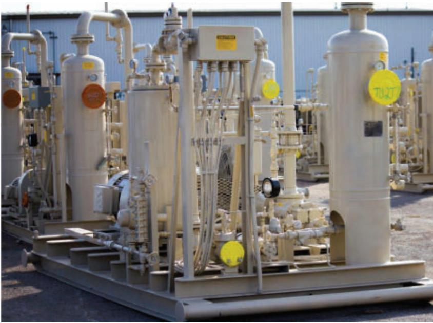
■ HY-BON builds, repairs and packages rotary vane, reciprocating and screw compressor VRU packages. Low-maintenance, standard units are staged and ready for immediate delivery for new tank vapor recovery applications.
