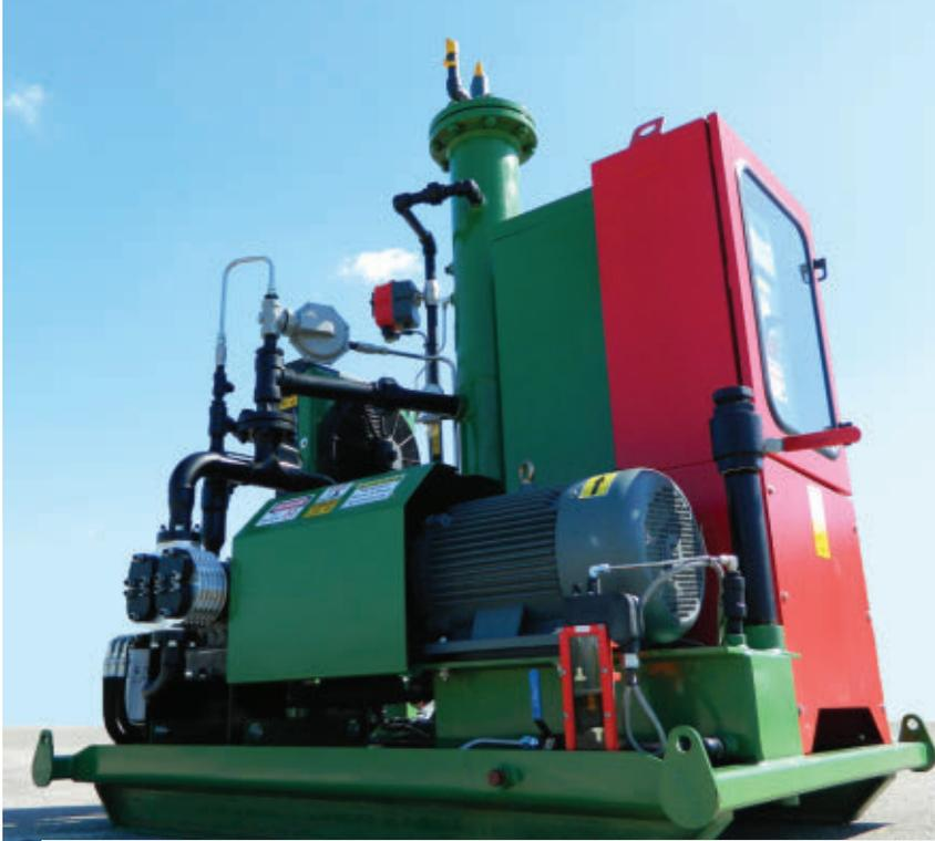
■ This standard zero-emissions GTO-20E package is OTA Compression's top-selling VRU. It features the company's proprietary KS40 reciprocating compressor driven by a 20 hp (14.9 kW) electric motor equipped with a VFD.
